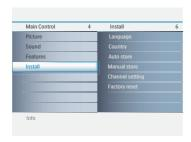
Auto Store: to start automatic search for all programmes available in your region. If the transmitter or cable network sends the automatic sort signal, the programmes will be numbered correctly. If this is not the case, you need to use the Channel setting menu to renumber the programmes.
